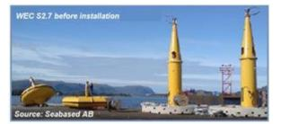
in the form of blasting or excavations are not necessary. Deployment of the WECs on the seabed protects them from extreme conditions that may occur at the surface of the sea and helps minimize required maintenance. From the point of view of maintenance operations, an individual WEC can be disconnected and replaced without affecting the function of other parts of the wave park, which
