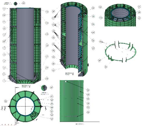
Figure 3. OCEANTEC oscillating water column floating device
