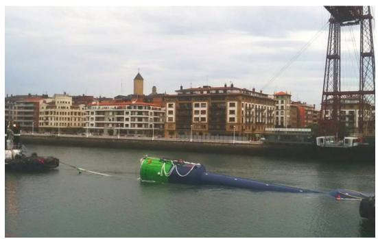
Figure 6. Towing of the OCEANTEC vertical floating device
