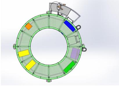
Figure 4. OCEANTEC oscillating water column floating device - top view
